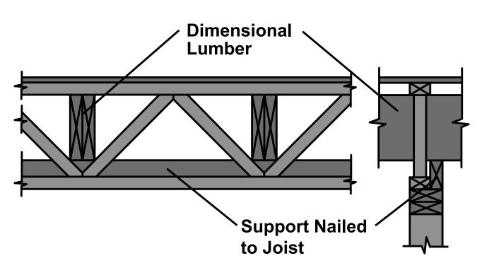
NOTE: Cantilevered Dimensional Lumber Must be Engineered for Load and Deflection Per Applicable Code
