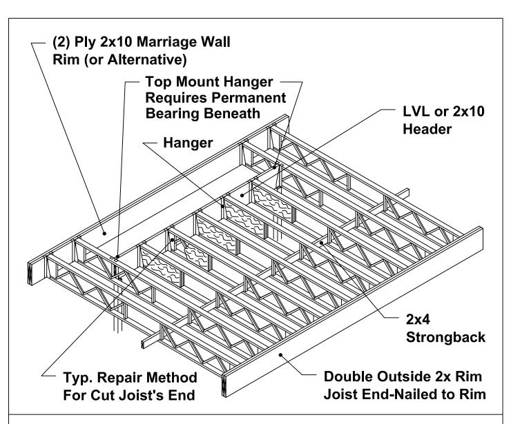
STAIRWAY OPENING PERPENDICULAR TO FLOOR JOISTS (CENTER CHASE OPENINGS ALIGNED)
